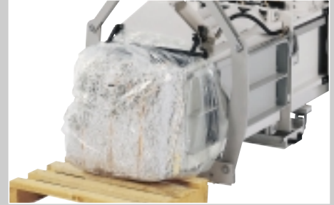
Semi-automatic bale strapping, bales can also be pressed directly in a plastic sack.
